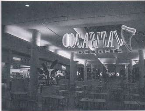
Figure 13-12. Whimsical signage delineates the food court of an upscale mall. A variety of light sources contributes to the cheerfulness of the place, including neon, fluorescent, and metal halide. Daylighting is incorporated through a skylight and window walls.
