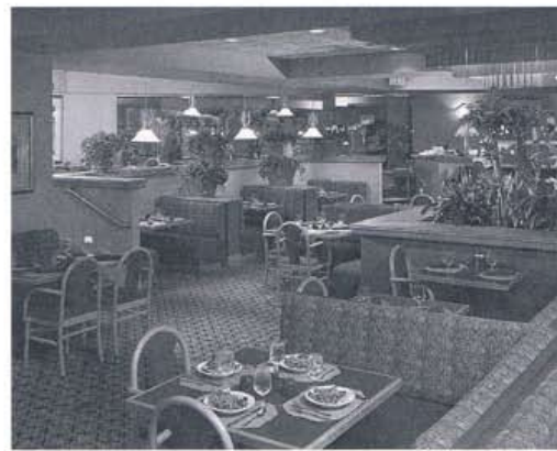
Figure 13-11. This hotel restaurant has a cheerful interior with a moderate illuminance level. Pendant luminaires delineate the section of booths.
