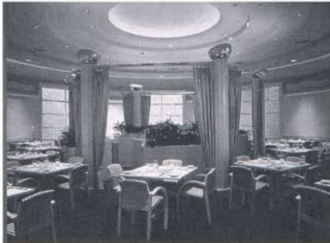
Figure 13-10. A circular design element is used in a number of ways in this intimate restaurant: in the concentric circles in the ceiling, in the circular cove lighting, and in the circular waiting area that can be set off from the dining area by draperies. Downlights are aimed to illuminate table tops and provide general lighting.
