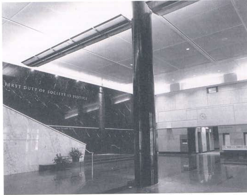
Figure 11-15. The main lobby of a building should provide a good impression. Materials in lobbies are often of high reflectance. The lighting should enhance the beauty of the building materials and at the same time minimize visible reflections.
